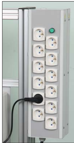
Sockets on the back of the console for connecting the modules
